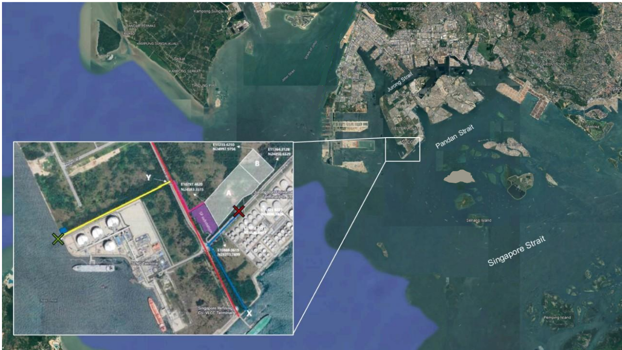
Figure 1-1 Proposed location of CCGT at Southern Jurong Island; intake point is indicated by yellow "X", and outfalls by red "X"
