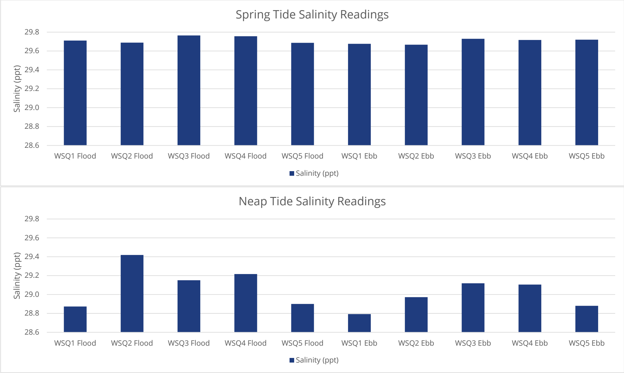
Figure 3-3 Average tide readings for salinity across spring and neap, flood and ebb tidal conditions at each sampling site.
